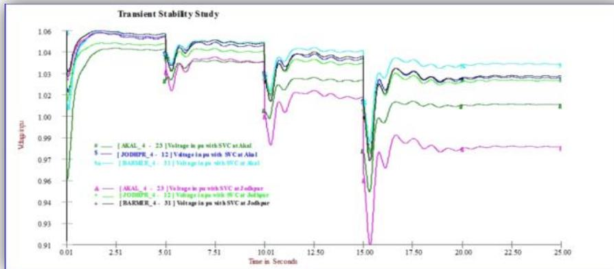
**Fig.19 Voltage at 400KV GSS with SVC location change**
