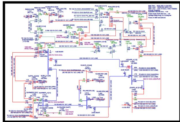
**Fig. 18 SVC at Barmer with full wind generation condition**
