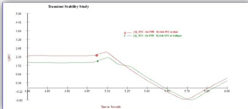
Fig. 28 SVC Q flow with LLLG fault condition
