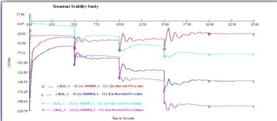
**Fig. 21 Reactive power flow variation in 400kV lines with change of location**
