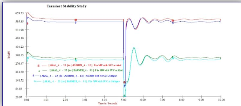
Fig. 26 Active power flow in 400 kV lines with LLLG fault condition
