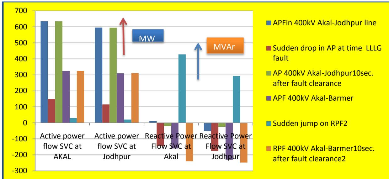
**Fig.37 Flow of active and reactive power in 400 kV Akal- Jodhpur and Akal- Barmer Transmission line under LLLG Fault at 400kVBarmer Bus**
