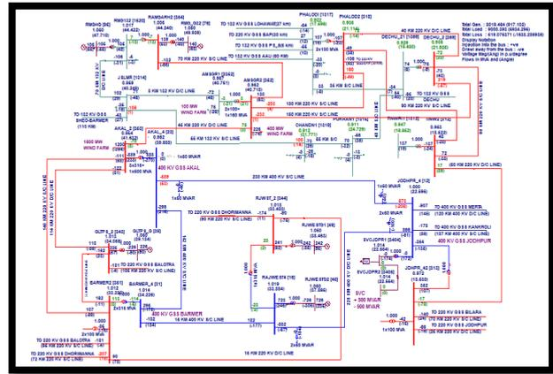
**Fig.17 SVC at Jodhpur with full wind generation condition**
