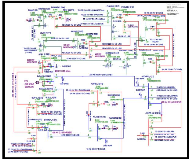
**Fig.11 Increase in wind power 50% with double circuit 400 kV Akal Jodhpur and Akal Barmer line**
