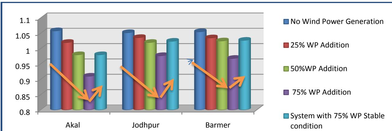
**Fig.35. Bus Voltage & Voltage dip with the addition of WP with SVC installed in Jodhpur**
