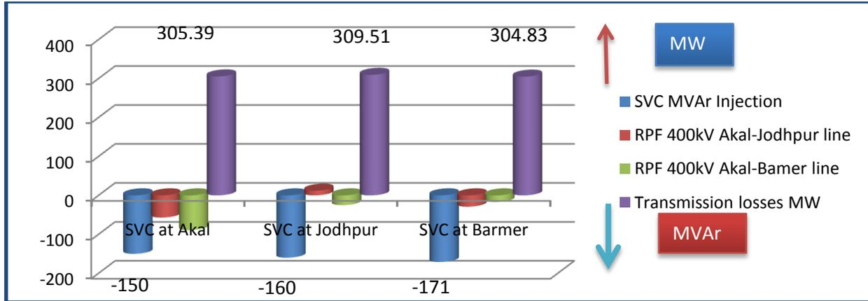
**Fig.31 Reactive power injection by SVC, reactive power flow in 400 kV Lines & transmission losses due to change of location of SVC at no wind power condition**
