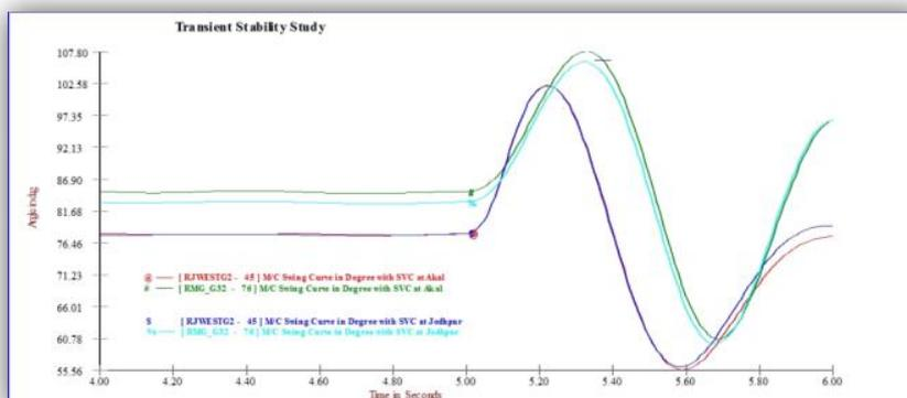
Fig. 29 Swing performance of power plants with LLLG fault condition
