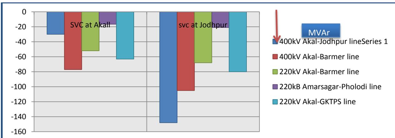
**Fig.36. Flow of reactive power in 400&220 kV Transmission lines with SVC installation at Akal and Jodhpur**
