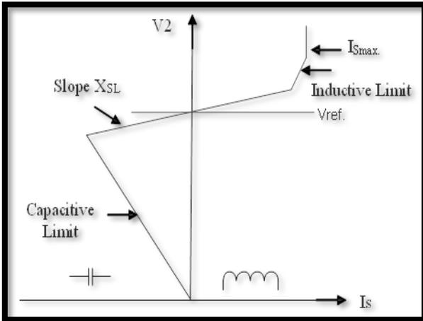
Fig.1. Steady state V-I characteristic of SVC
