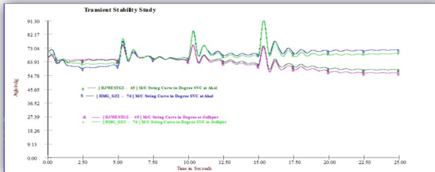
Fig.24 Swing curve of M/s Raj West & Ramgarh PP with change of location of SVC
