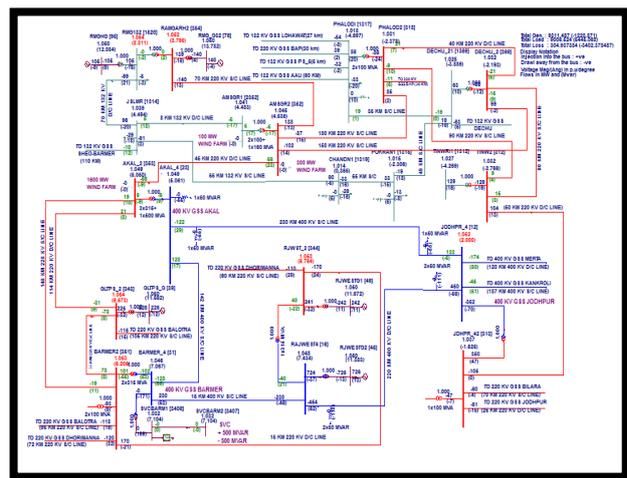
**Fig.15 SVC at Barmer with no wind power condition**
