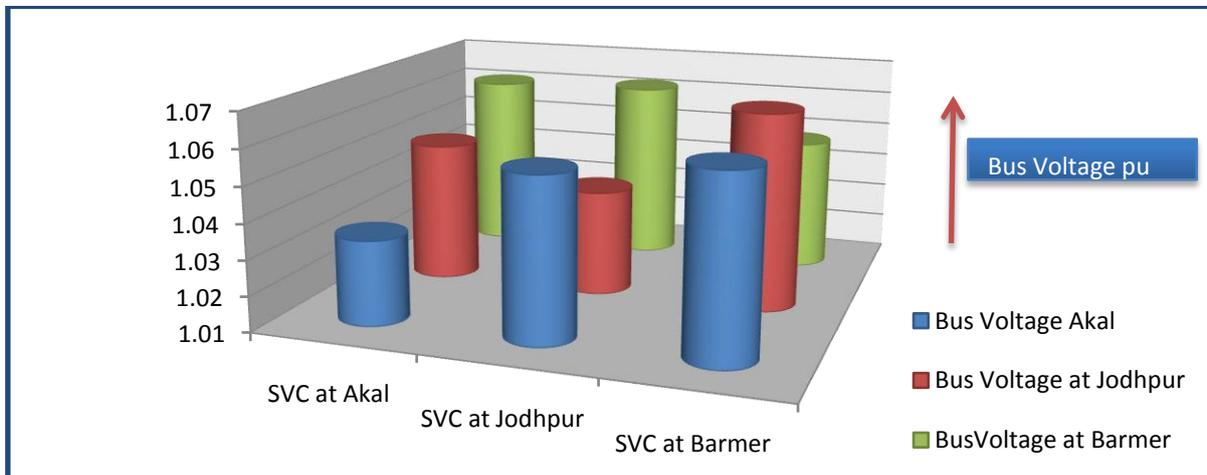
**Fig.30 Bus voltage under steady state conditions at different 400 KV GSS due to change of location of SVC at no wind power condition**
