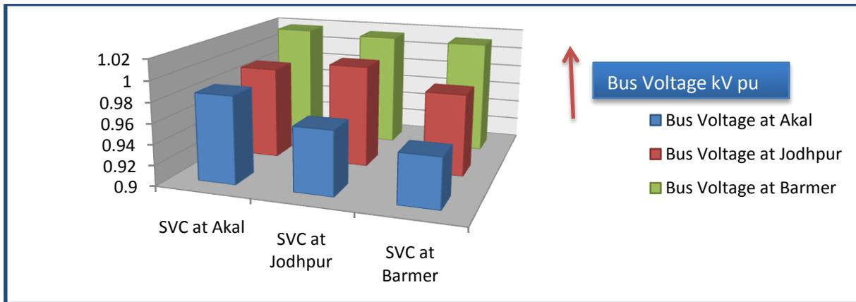
**Fig.32 Bus voltage under steady state conditions at different 400 kV GSS due to change of location of SVC at full wind power condition**
