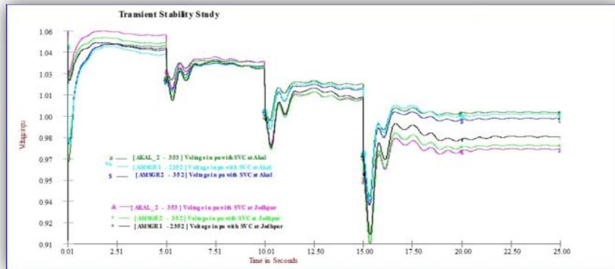
**Fig. 20 Wind bus voltages with SVC at Akal and Jodhpur**
