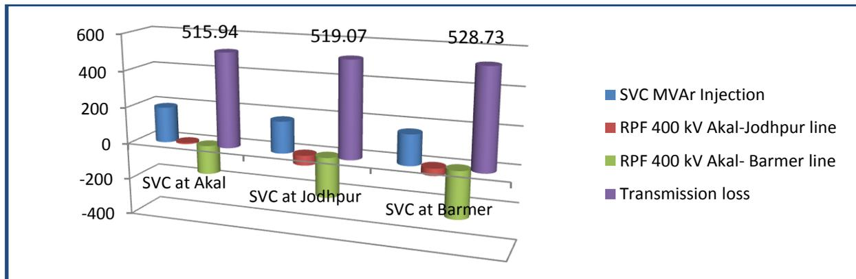
**Fig.33. Reactive Power Injection by SVC, Reactive Power Flow in 400 kV Lines & Transmission Losses Due to change of location of SVC at full wind power condition**
