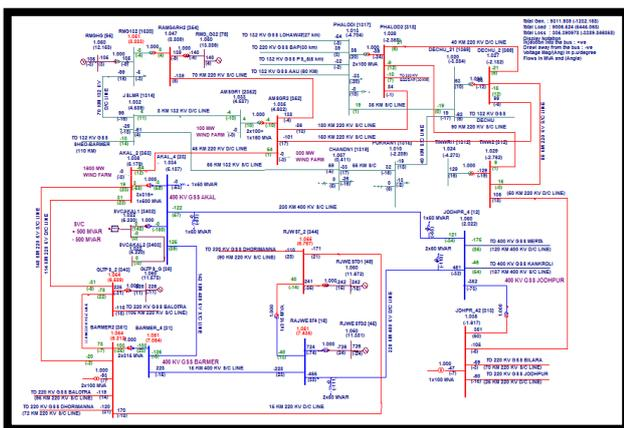
**Fig.13 SVC at Akal with no wind power condition**
