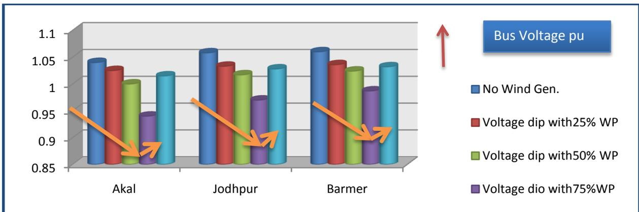
**Fig.34. Bus Voltage & Voltage dip with the addition of WP with SVC installed at Akal**
