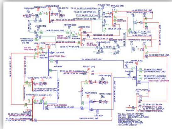
**Fig.4 Power plot with minimum load and wind power generation**
