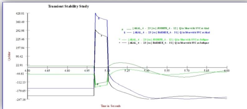
Fig.27 Reactive power flow in 400 kV lines with LLLG fault condition
