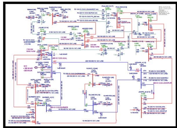
**Fig. 7 Increase in wind power penetration 10%**
