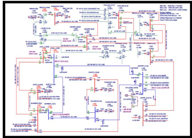
**Fig.14 SVC at Jodhpur with no wind power condition**
